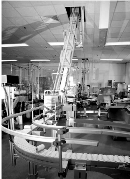
Figure 4.13. Chain conveyor: Flexible link conveyor for light piece goods (Carrying chain conveyor) [Photo: FLEXLINK]
