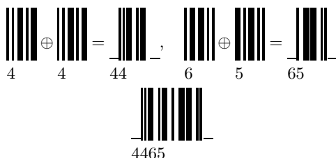
Figure 6.7. The number 4465 in code 2/5 interleaved without start and stop character and without check digit
